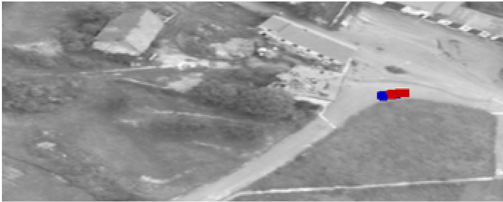
Figure 9: Detected moving objects: red and blue color denote position change of detected object in a given image pair.
